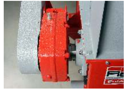
Belt drive – spur gear reduction
